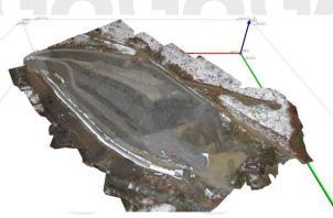
3D images from drones are a perfect survey of large blast sites. Poor blasting results are often caused by inaccuracy of the front row hole placement and inaccurate blast pattern geometry.
